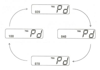
When finished, press MEM to store onto memory. The displayed Tone Period stops flashing and three successive beeps will be heard. Press TSQ for about 1.5 seconds to exit. The radio returns to normal operation. Or press TSQ momentarily to go to the next programmable parameter.
